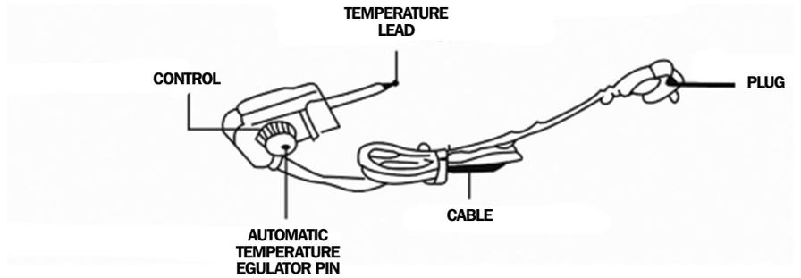
1. The automatic temperature regulator is a highly sensitive part, you must be very careful not to damage the part in any way.
